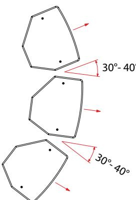
Correct positioning of the cabinets: an angle within 30° / 40° minimizes horns interaction and gives a linear frequency response.
