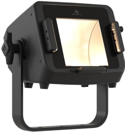
The **EclExpo Flood150** is a compact, bright, and versatile floodlight that is designed to be a substitute for traditional CDM, HMI, and tungsten small floods in tradeshows, theaters, or as a work light. Just like its classic predecessors, but with a custom LED source, this unit features a linear light source combined with a reflector, which ensures a wide coverage of 100° (Horizontal) x 60° (Vertical) of indirect light emission.
