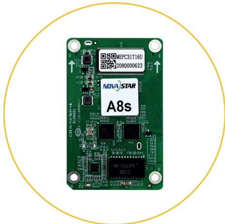
Novastar A8S Receiver Card
