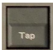
The Tap button is used in conjunction with the Tap Tempo feature within Ai. Turn on the Tap Tempo widget in Ai either from within the software or using the Tap Widget function button on the Sapphire, then hit the Tap button four times to set the tempo you wish to work with.
