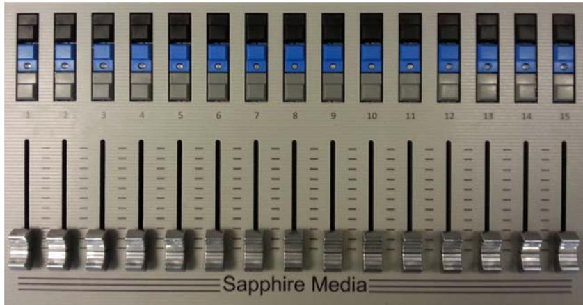
Using the Avolites Controller Template Project (found in the project browser of Ai), the Sapphire's 15 faders refer to the currently active row on the Roller Cue and allow the user to trigger and fade in media on the selected layer and fixture.
