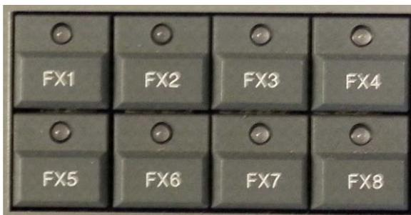
These buttons are assignable and designed to be used to trigger effects.
