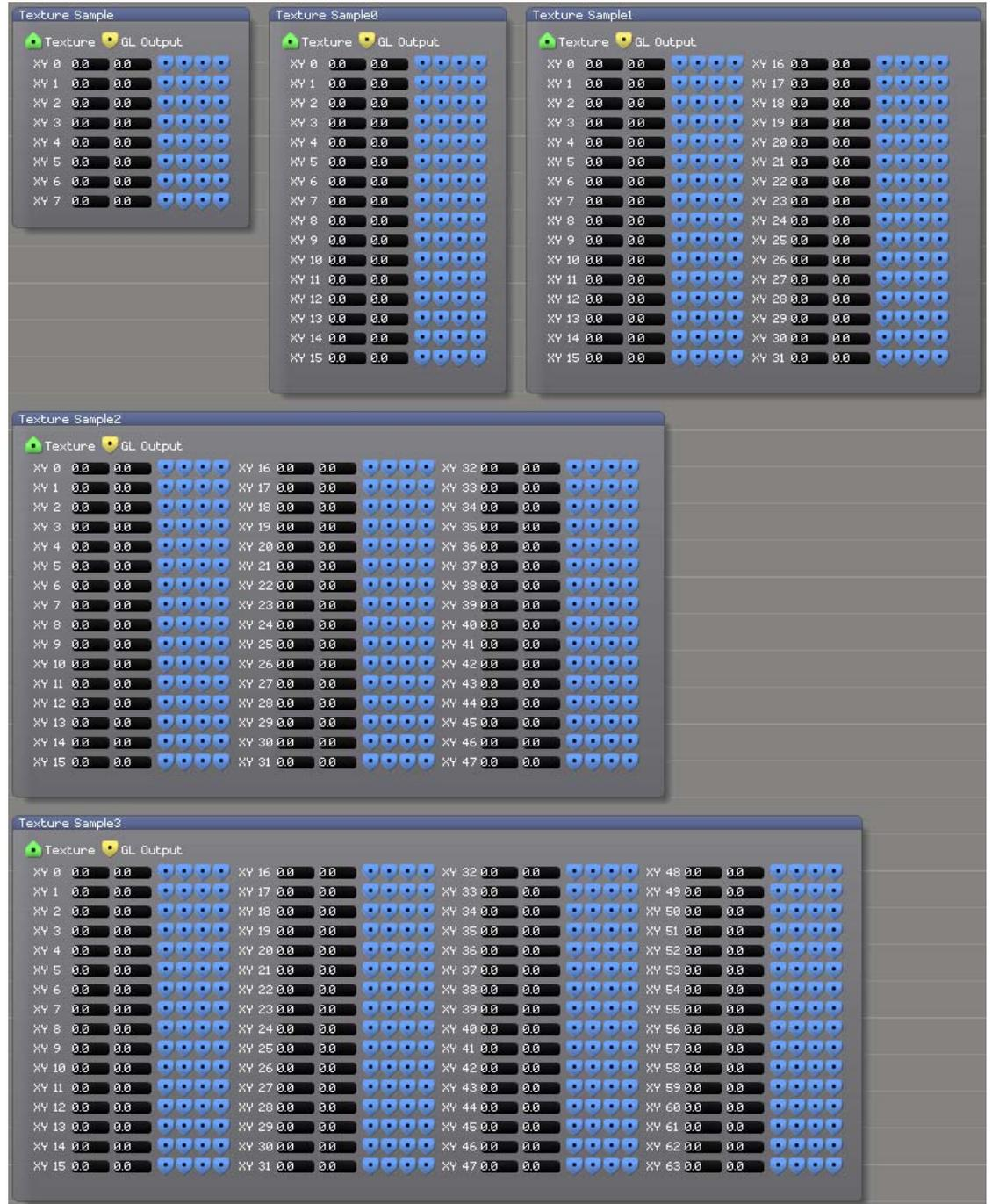
Allows sampling of an RGBA texture connected to the Texture port. The GL Output port should be merged with an active render path. Up to 64 Locations can be specified in X and Y pixel coordinates and the corresponding RGBA colour information will be output on the adjacent controller ports.
