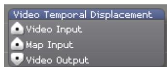
Adjusts the temporal play back of the video received at the input and outputs the resulting video signal.
