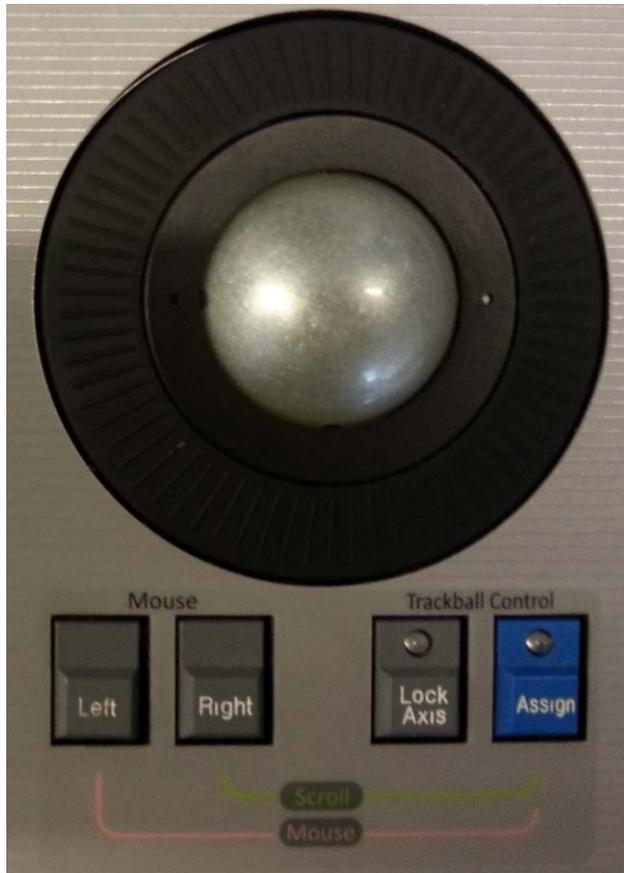
The trackball and mouse controls allow the user to navigate Ai without the need for an external mouse. To activate the trackball simply press and hold the Assign key then press the Left mouse button.
