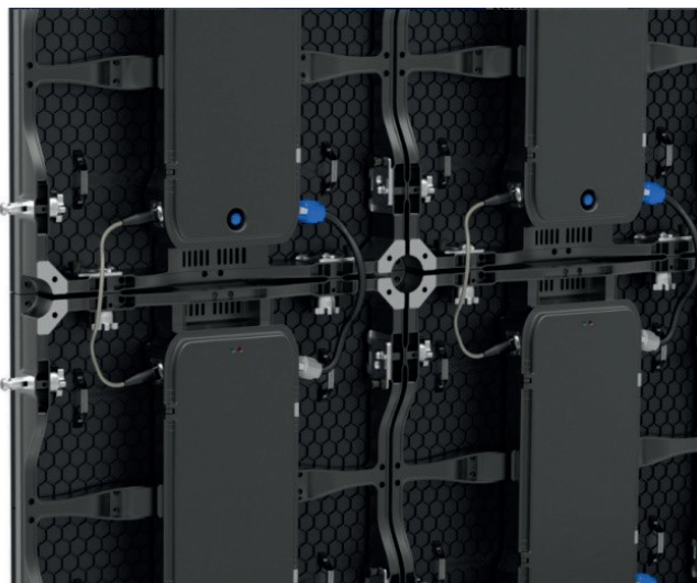
Image 4-7 Two tiles vertically connected with side lock
