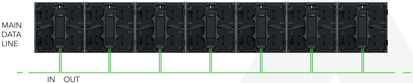
**NOTE:** it's suggested to distribute the signal as evenly as possible between the various signal lines
