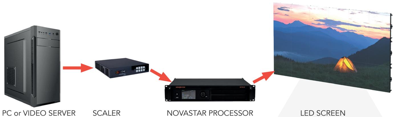
Novastar processor is the sending card that sends signal to cabinets. Each cabinet has a receiving card mounted in. Novastar processor has a different number of DATA output depending from the product version. Each DATA output can manage a max number of **650.000 pixels**.
