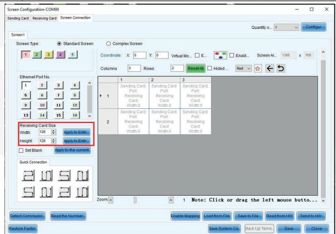
**7** Select the port of the processor and draw the data line on the screen (view from behind)
