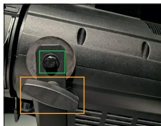
3) Unscrew the noted screws to remove the metal plate from both sides of the fixture
