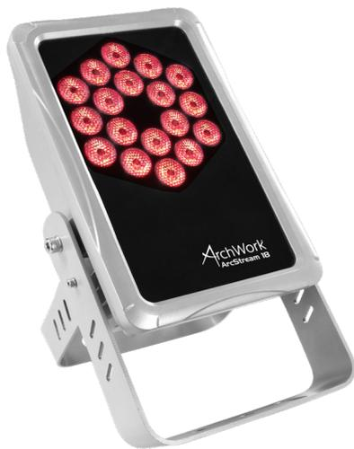
**ArcStream 18** is a professional architectural colour-washer conceived to house 18x3W RGB/FC LED in a single matrix. The projector is built inside a super-slim aluminium case which allows an IP65 protection rating for outdoor lighting projects and provides homogeneous colour synthesis even on short distance. **ArcStream 18** employs a touch-capacitive display to arrange settings in a quick and easy way without the external coder.
