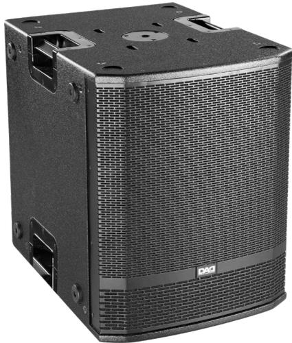
Active subwoofer, D-class amplifier, 1000W, 133db SPL. The BX18SA is an 18" powered subwoofer that provides a powerful low frequency response. The geometry of the reflex duct is low compression thanks to the aerodynamic development. This design guarantees precise and well controlled bass response even at high volume.
