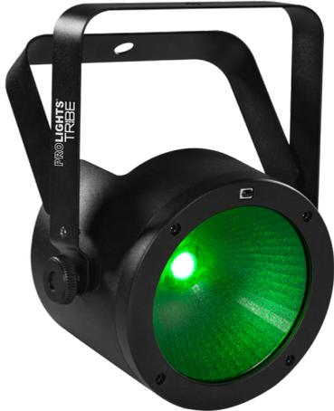
**FlatCob 40** is a compact LED projector equipped with a COB source that allows for placement of a bright RGB/FC 40W LED in a super-slim housing. The light source features 60° beam angle with a magnetic lens holder (included) to switch the projection at 30°. **FlatCob 40** can be controlled wirelessly through the optional USB WIFI transceiver in combination with WIFIBOX and the SmartColor app or through IR remote.
