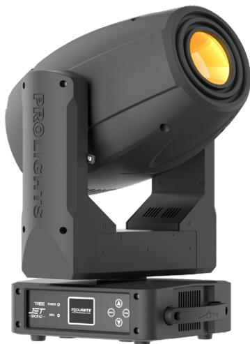
**Jet Spot4Z** is a 180W 6.800 K LED spotlight designed to replace a 700W discharge fixture in theatres, concert halls and a host of other venues. The compact size allows for the use of this luminaire in venues with low ceilings without resorting to zoom. Its custom optical system delivers a consistent output with a flat-field and crisp gobo projection right through the massive 11° to 38° zoom range.
