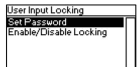
When pressing the [OK] button from the Home Screen of a locked device, it will prompt for the password. If it is entered correctly, the device becomes unlocked and the main menu is displayed. A padlock symbol in the top right corner of the Home Screen indicates that the user input is currently locked.
