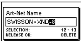
Then keep [OK] pressed and turn the encoder clockwise until all of the text that you wish to delete appears highlighted.
